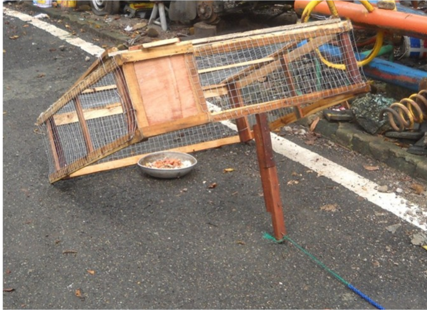
Figure 1. The Drop-trap made of light weight, sturdy wood covered with a 1 in x 1 in chicken wire mesh. The dimensions of 3 ft x 3 ft x 14 in (L x W x H) propped up by a 16-in stick connected to a string. A small, sliding wooden door of 7 in x 18 in (W x H) was placed to facilitate transfer of animals into portable cages.
