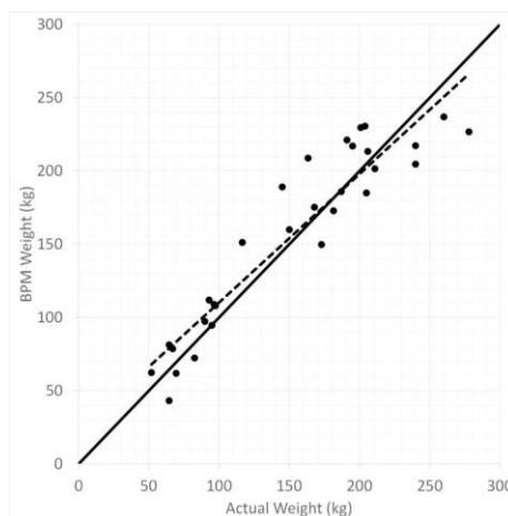
Figure 6. Plot of estimated live weight using pixel-based (dashed line) to perfect linearity (solid line).
