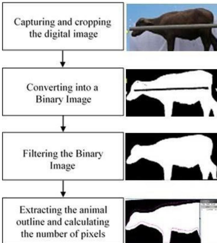
Figure 3. Image process flow diagram for calculating lateral body surface area using ImageJ.
