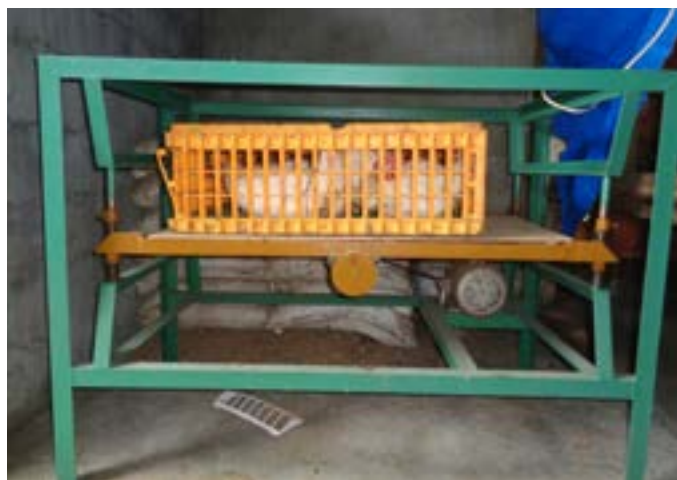
Figure 1. Vibration simulation set-up of the experimental birds consists of a table on soft springs with actuating system that included adjustable weights on two counter rotating shafts (counterweights), that revolves in opposite directions at the centre of gravity of the table and its load, providing vertical vibration. Because the frequency of the vibration simulator table is counterweights, the frequency of the table was obtained based on the number of revolutions of the electric motor.
