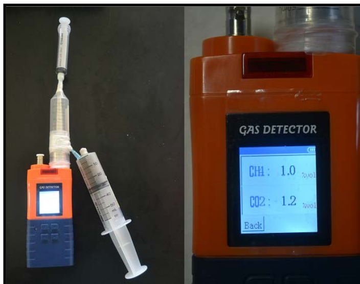
Figure 2. Non-dispersive infrared gas detector used to quantify methane and carbon dioxide from the in vitro gas production of rumen fluid from cattle with different diets. Sensitivity: parts per thousand
